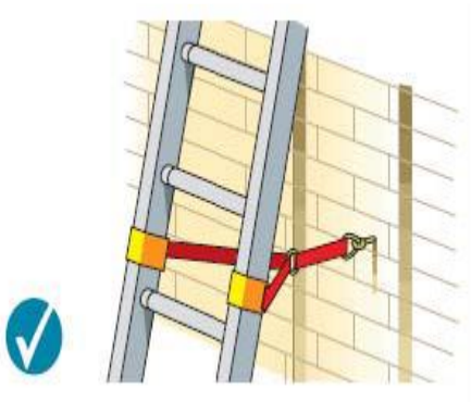
Tying near the base
